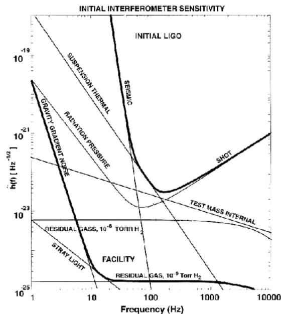
Figure 4: The different disturbances of the interferometer[5]
