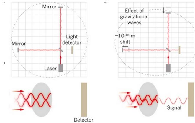
Figure 3: The two different results of combined light beams[3]
