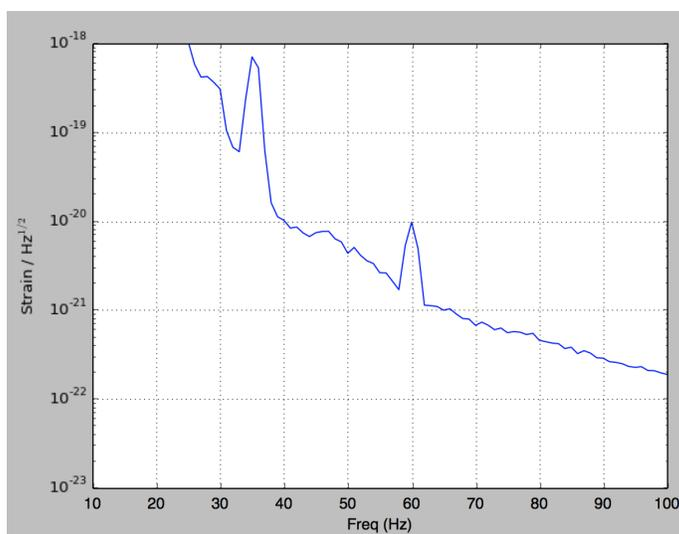
Figure 5: The ASD plot of a random LIGO file, including a distinct strain peak at 60 Hz
