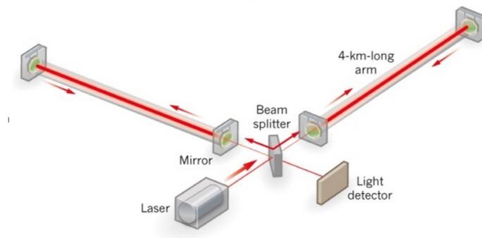
Figure 2: A brief description of the structure of the LIGO detector [3]
