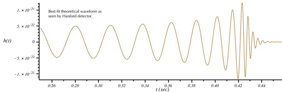
Figure 2: gravitation “CHIRP” caused by rotating pair of massive objects; note the increasing amplitude and frequency as a function of time <sup>[3]</sup>
