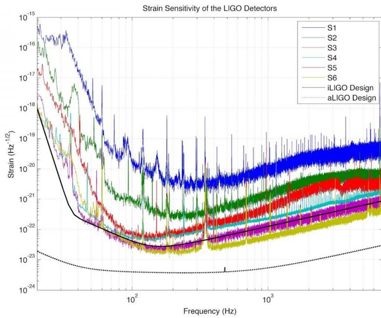
Figure 5: The improvements in LIGO’s sensitivity over the several scientific runs and how they approach the initial target sensitivity of LIGO
