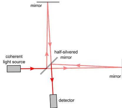
Figure 3: the basic structure of Michelson Interferometer [5]
