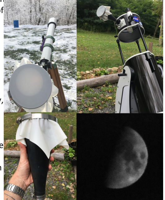
Sun Funnels in action! Starting clockwise from the bottom left, a standalone Sun Funnel; attached to a small refractor to observe the transit of Mercury in 2019; attached to a large telescope in preparation for evening lunar observing; projection of the Moon onto a funnel from a medium-size scope (5 inches). Safety tip: NEVER use a large telescope with a Sun Funnel to observe the Sun, as they are designed to project the Sun using small telescopes only. Some eager astronomers have melted their Sun Funnels, and parts of their own telescopes, by pointing them at the Sun - large telescopes create far too much heat, sometimes within seconds! However, large instruments are safe and ideal for projecting the much dimmer Moon. Small telescopes can't gather enough light to decently project the Moon, but larger scopes will work.
